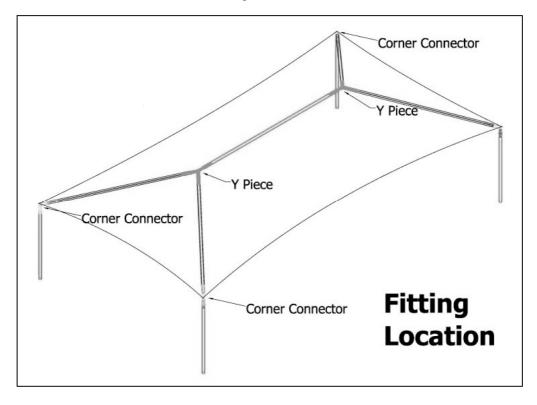
• The whole top structure is now self supportive and no further support from the ladder is required. Ensure that all tubing is fully inserted up to the stopper.
